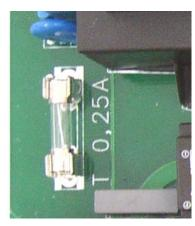
The electronic control system is protected by a 0.25A fine-wire fuse on the PCB in the inside of the device. The short-circuit protection for the filter pump must be provided by a backup fuse of maximum 16A on site.
