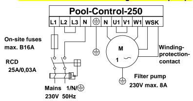
The bridge fitted in the works between the terminals labelled WSK must be removed if a pump with coil earthing contact is connected. If no such connection is made, it must remain fitted. These terminals carry mains voltage!
